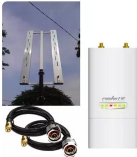
Gambar 3.4. Contoh access point wireless outdoor.
