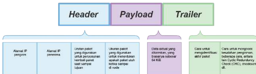
▲ Gambar 4.5 Struktur Paket (Packet Header, Packet Payload, dan Packet Trailer)
